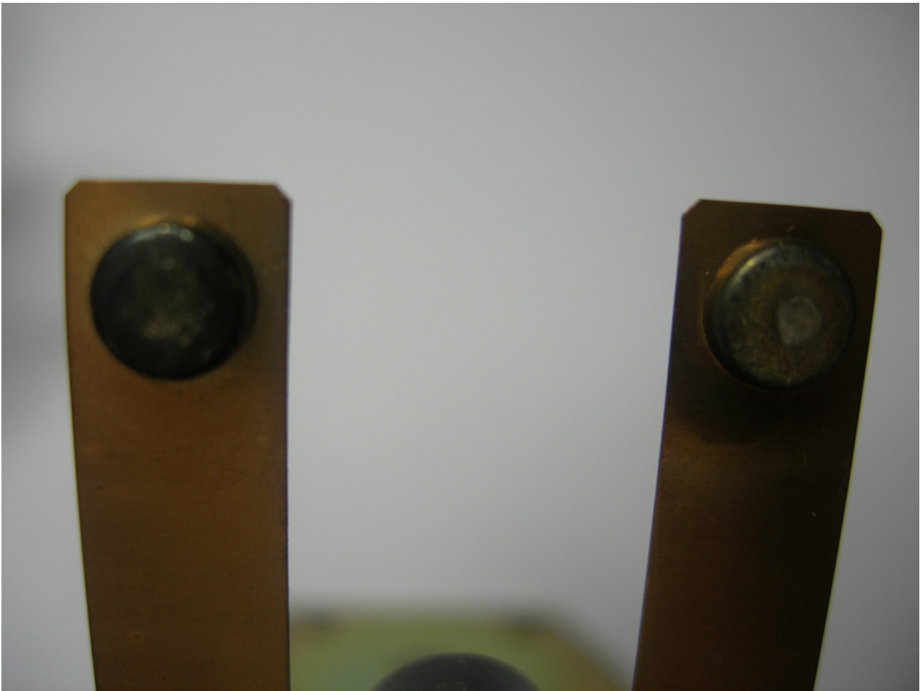
Fig. 4 –Another view of the contacts of the relè
